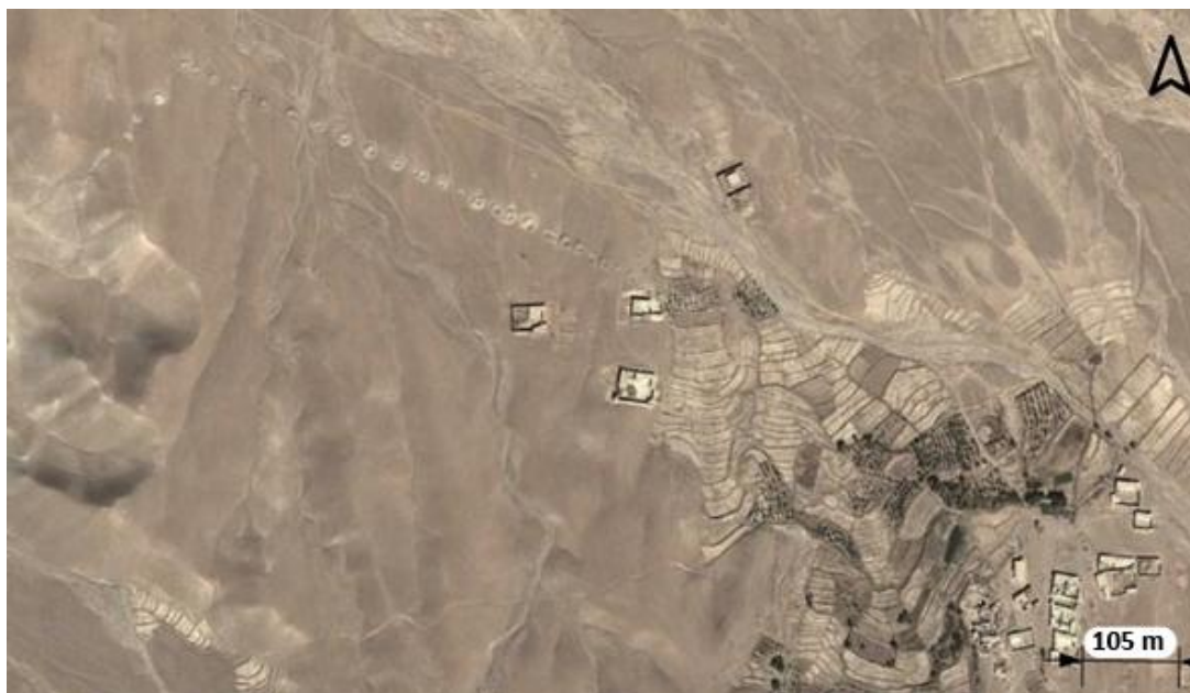
Figure 3. Typical karezes in Afghanistan identifiable as chains of light-color spots (Google Earth, 2020).
