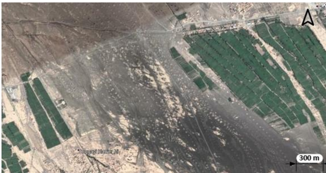
Figure 4. Karezes in the Turfan Depression, China, identifiable as long chains of light-color spots (Source: Google Earth, 2020).
