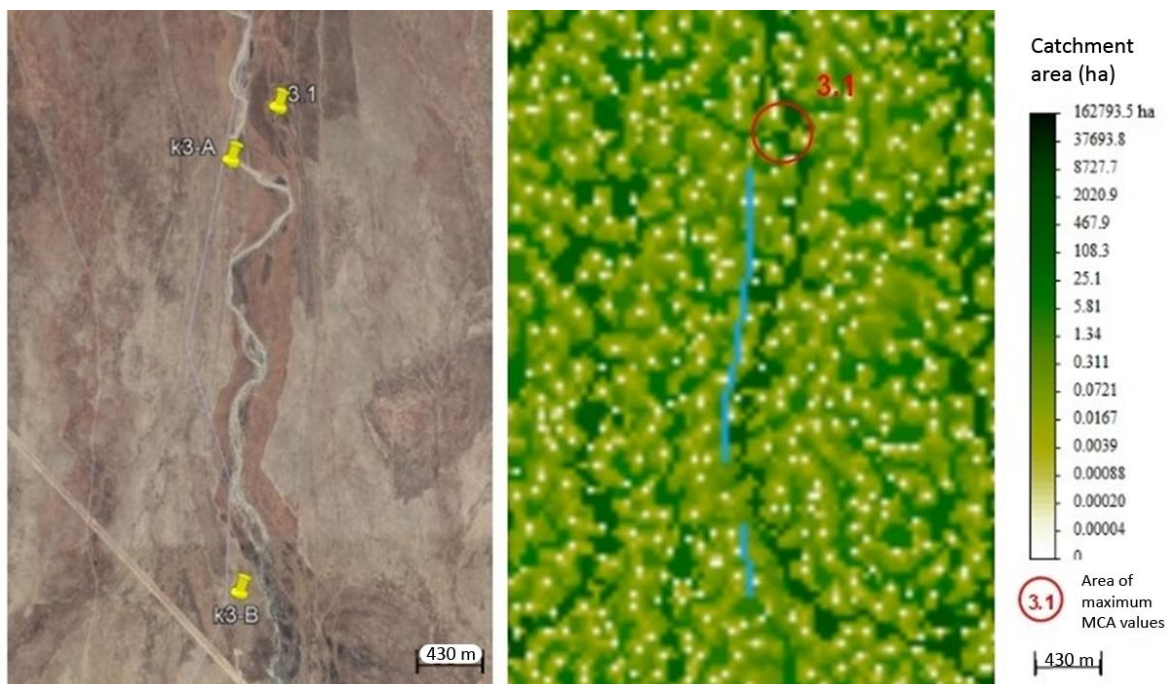
Figure 8. Karez №3 on the satellite image (Google Earth, 2020) and MCA map (k3-A and k3-B correspond to karez start and end points; number 3.1 correspond to maximum MCA values around the mother well).
